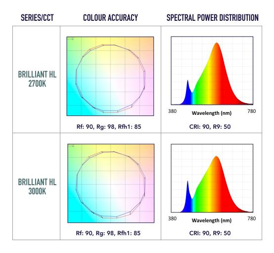
Rf: TM-30 metric measuring colour fidelity (whether colours are similar to those under natural light). Rf is a more accurate version of the CRI Ra. Rf is 100 for natural light. Rg: TM-30 metric measuring colour gamut (whether colours are more saturated than under natural light). Rg is 100 for natural light. Rfh1: TM-30 metric measuring colour fidelity for red tones. Rfh1 is a more accurate version of the CRI R9. Rfh1 is 100 for natural light.
