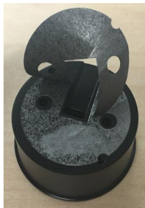
Figure 3: Black protective liner removal from SLC thermal graphite pad
