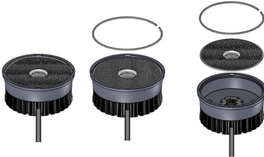
Figure 2: Lens attachment with circular spring-clip
